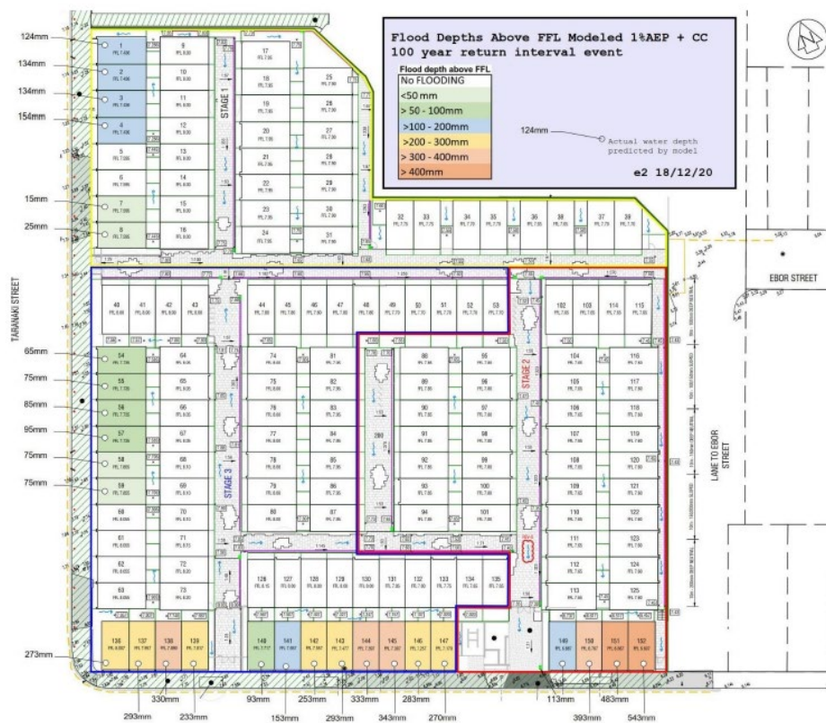
Figure 4: Projected flood depths in mixed-use units
