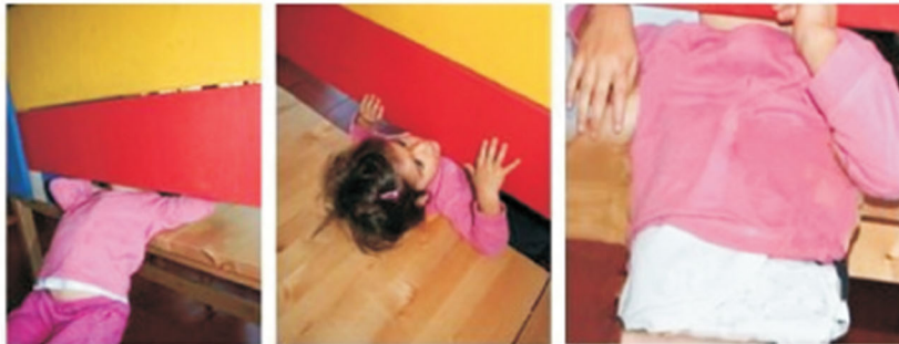
Figure 1 - A gap of 11 cm allows the child's body to pass entrapping the head.
