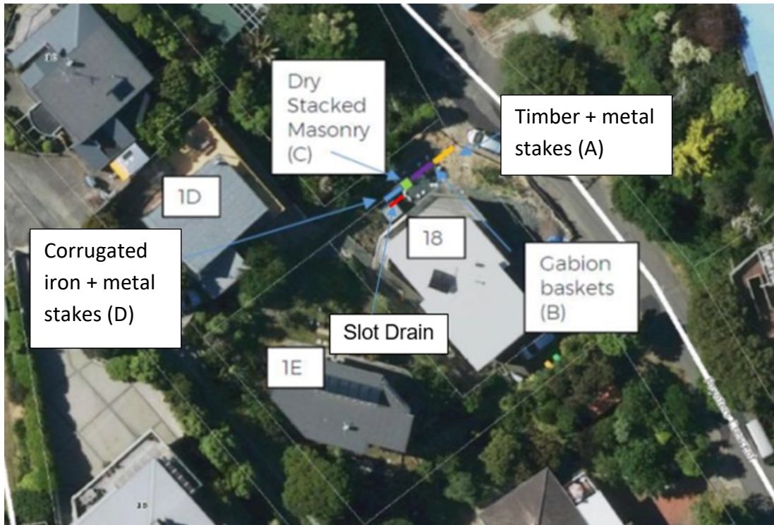
Figure 6: Plan of approximate location of structures A (shown in yellow), B (shown in purple), C (shown in green), and D (shown in blue), and the slot drain (shown in red) [Not to scale]
