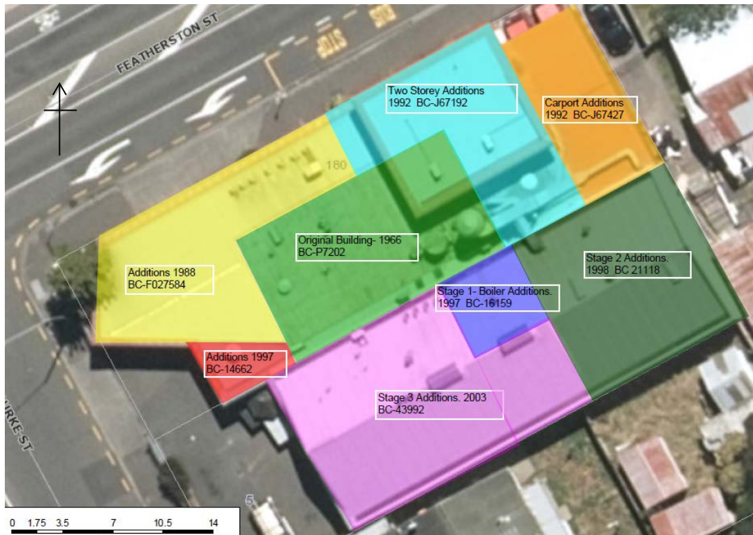
Figure 1: Aerial view 8 showing the building additions and the relevant building permits and consents
