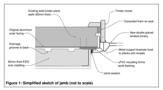
2.5 Given the date of construction in the 1970's, I consider the solid timber planks to external walls of the original house would have been boron-treated to a level that would provide resistance to fungal decay. The second expert was unable to verify the treatment of framing used in the small office addition.
