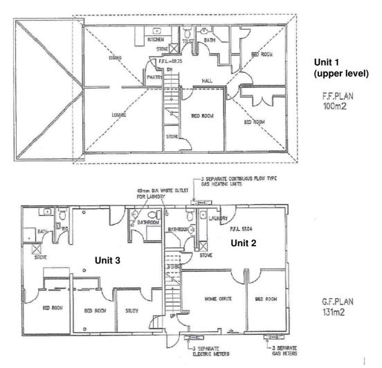
Figure 1: Floor Plan for the building (not to scale)
