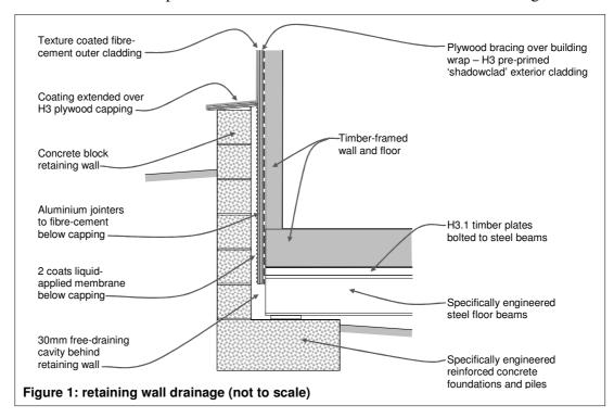
2.5 The architect has stated that the external wall framing is H1 treated. However, given the lack of evidence and the date of framing in 2002, I am unable to determine the particular level and type of treatment described as 'H1'; the wall framing of this house may not be treated to a level that will provide resistance to fungal decay.
