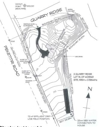
Figure 1: Site plan (not to scale)
