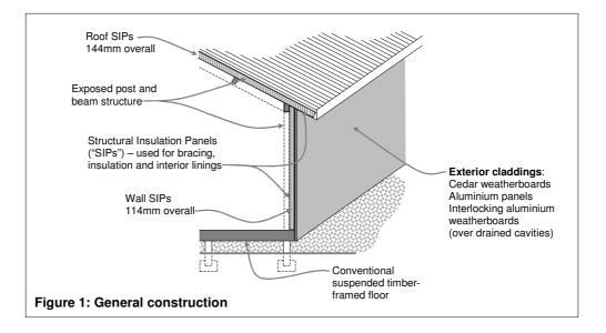
2.3.2 The exposed glue-laminated posts and beam structure of the house consists of 112mm x 112mm posts spaced at about 3.6m, which support 240mm x 90mm roof beams, with intermediate 190mm x 90mm rafters between. Bracing is provided by 'structural insulation panels' ("SIPs") as sketched in Figure 2.
