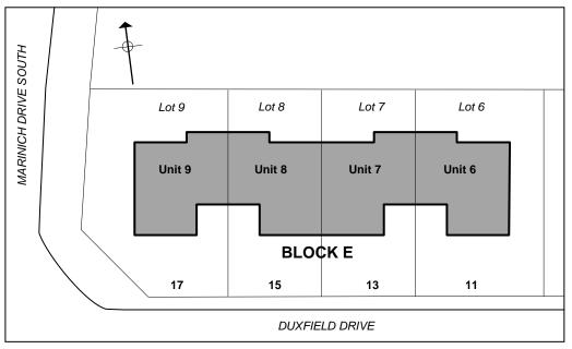
3.2 Block E is a two-storey building, which is situated on a flat site in a low wind zone in terms of NZS 3604<sup>3</sup>. The block sits at the corner of Duxfield Drive, with the main entries and garage doors facing south towards the road. The building is fairly simple
