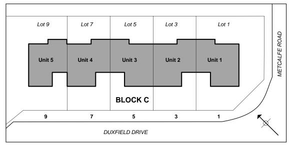
3.2 Block C is a 2-storey building, which is situated on a flat site in a low wind zone in terms of NZS 3604<sup>3</sup>. The block sits on the corner of Duxfield Drive, with the main entries and garage doors facing southwest towards the road. The building is fairly simple in plan and form, with garages set back from the front wall. The ground floor
