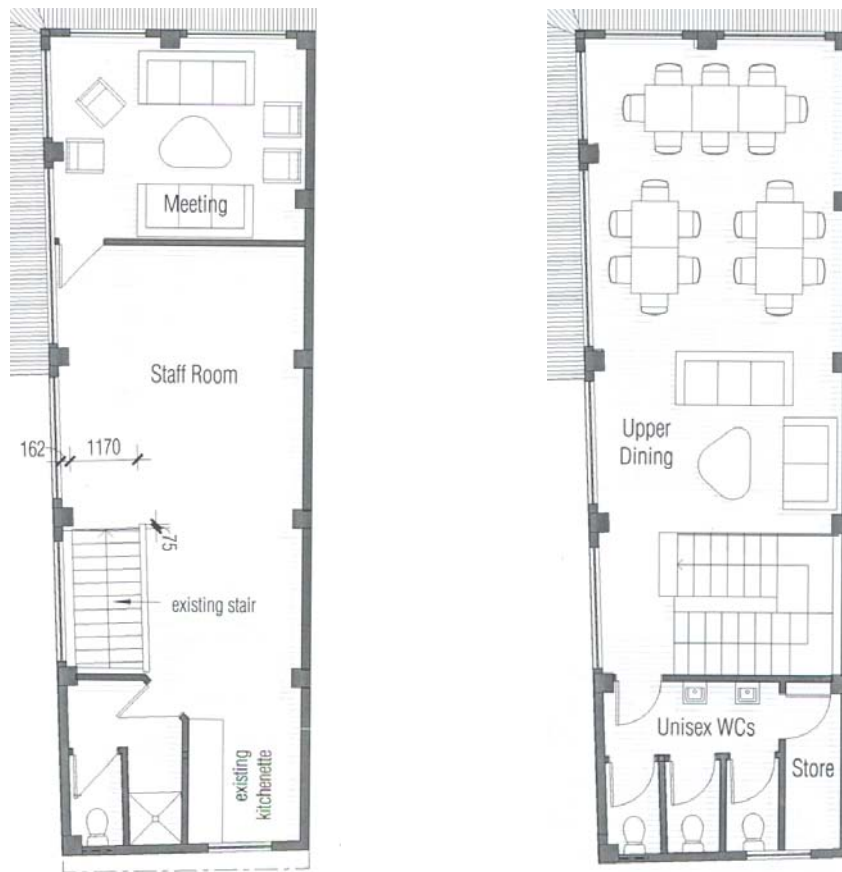
Figure 2: First floor plan as existing (left) and proposed (right)
