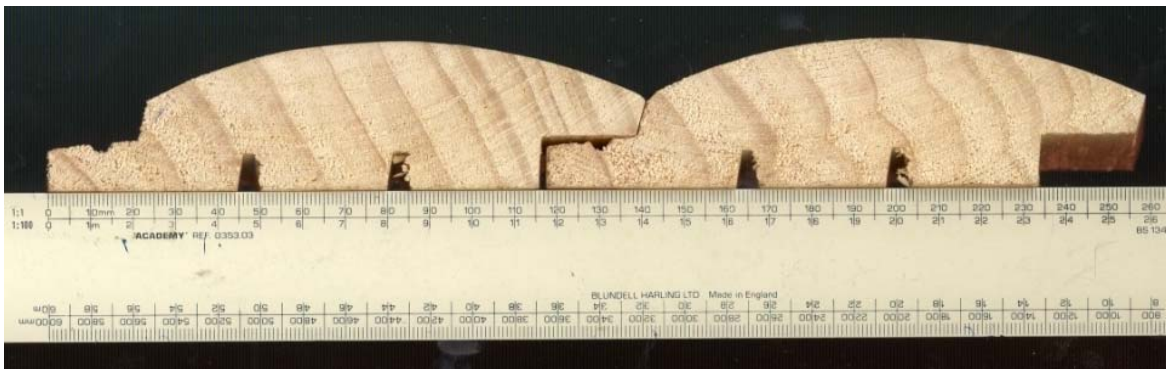
Figure 1: Cladding profile showing lapped joint
