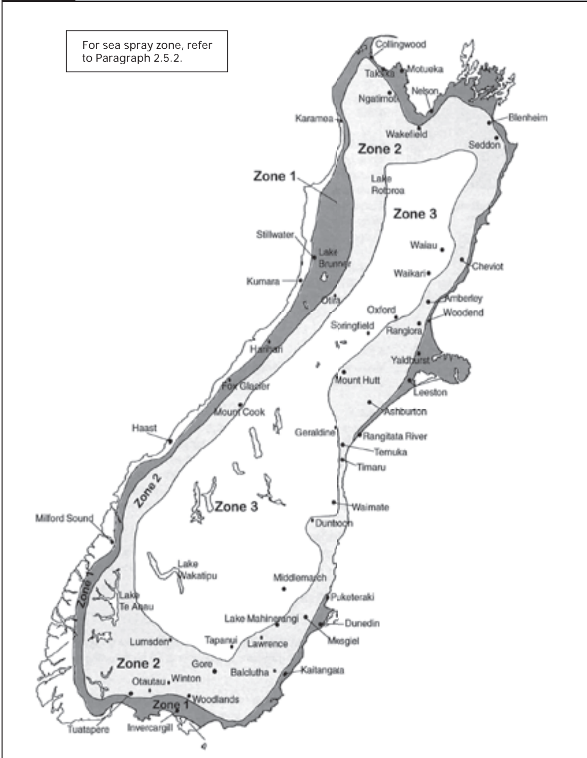
Figure 2.4 Corrosion zones – South Island Paragraph 2.5
