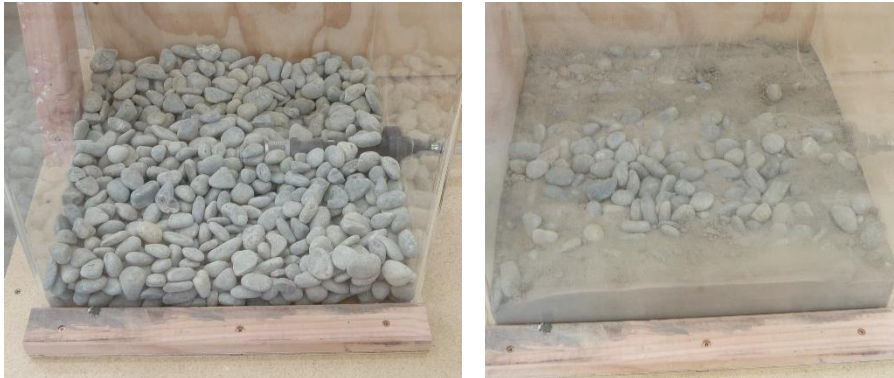
Figure 2. Tailings and fine sand (liquefaction material) layering
