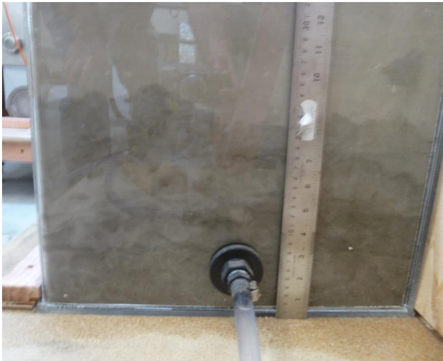
Figure 3. Water height visible in the column of tailings and sand mix
