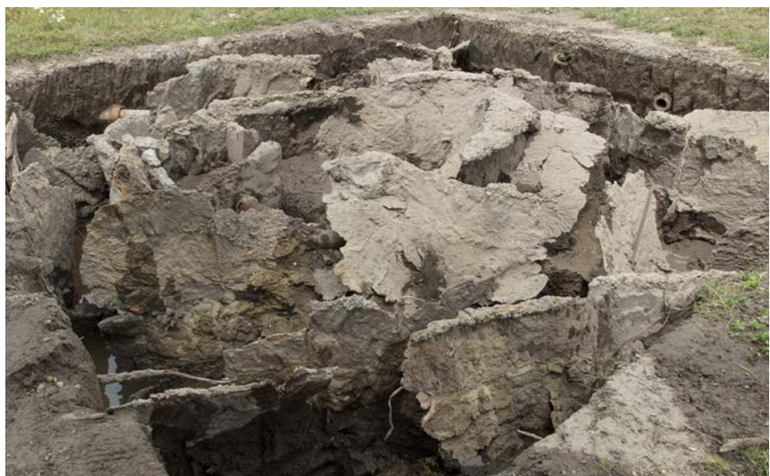
Figure 13: Hand-exhumed resin veins (left) and hydro-exhumed resin veins (right)
